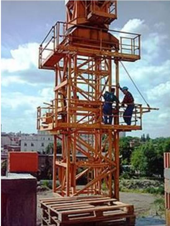
Self-erecting Tower Crane
